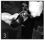
Use the tool provided to tighten the castor into place.
