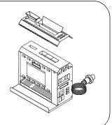
Install release sheet over platen. 12.7 mm (1/2") of release sheet should extend below platen on both sides of platen.
