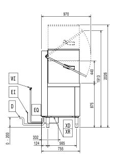
CWI1 = Cold Water inlet 1 (cleaning) XI = D Drain
